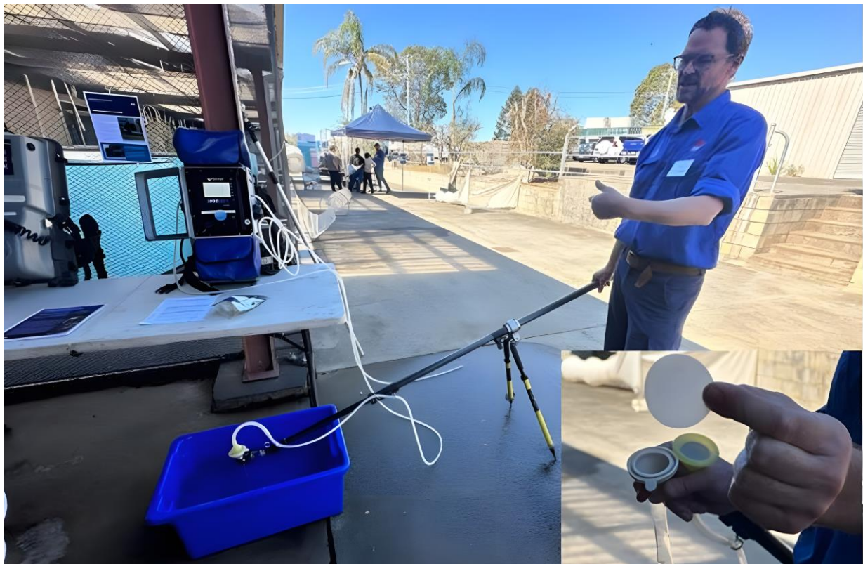
Sean demonstrating the E-DNA sampling pump. Particles trapped in special filters are later analysed for fish DNA.
